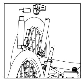
Install speed sensor and magnet on non-drive side of trike. Ensure wires are secure and clear of brake and steering components.
