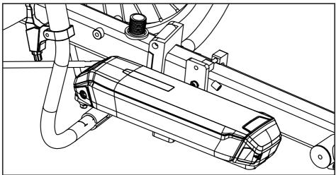
Install accessory mount and LED Remote onto handlebar. Refer to step 5 for wire routing.
