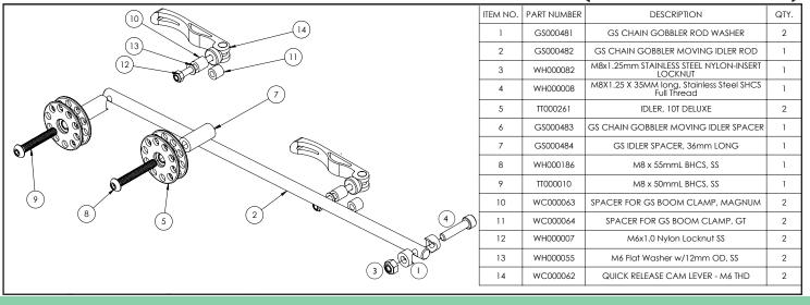
Remove boom clamp bolts. Install Quick Release Levers (14), Boom Clamp Spacers\* (10/11), M6 Flat Washers (13), and M6 Nyloc Nuts (12).
