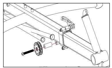
Install Moving Idler Rod Assembly on boom mount using the M8x35 bolt (4) and M8 Nyloc Nut (3).
