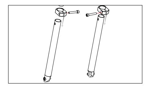
Attach rack and seat stays to seat frame using the M6x35 bolts, M6 washers, and M6 nuts.
