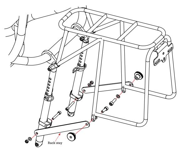
Adjust seat to desired height and angle. Level rack and secure 19mm clamp bolts.
