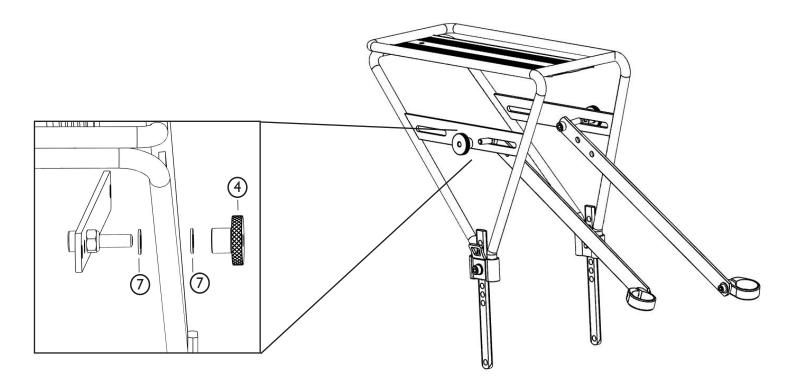
Loosen seat stay quick release levers and detach upper seat stays from lower seat stays. Loosen seat stay quick release set screws and remove clamps.
