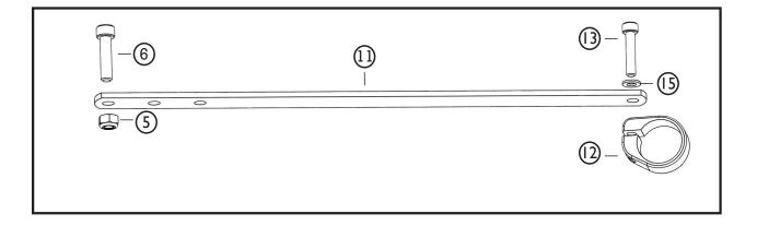
Attach rack stay assemblies to rear rack using the M6 thumb nuts. Leave thumb nuts loose for final adjustment. Note: Choose the appropriate rack stay mounting slot for best alignment with trike.
