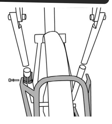
**Q** Level the Rack and tighten all fasteners.
