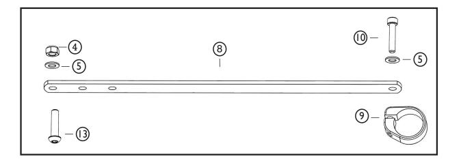
Attach rack stay assemblies to rear rack using the M6 flat washers and M6 nyloc nuts. Leave M6 nuts loose for final adjustment. Note: Choose the appropriate rack stay mounting slot for best alignment with trike.
