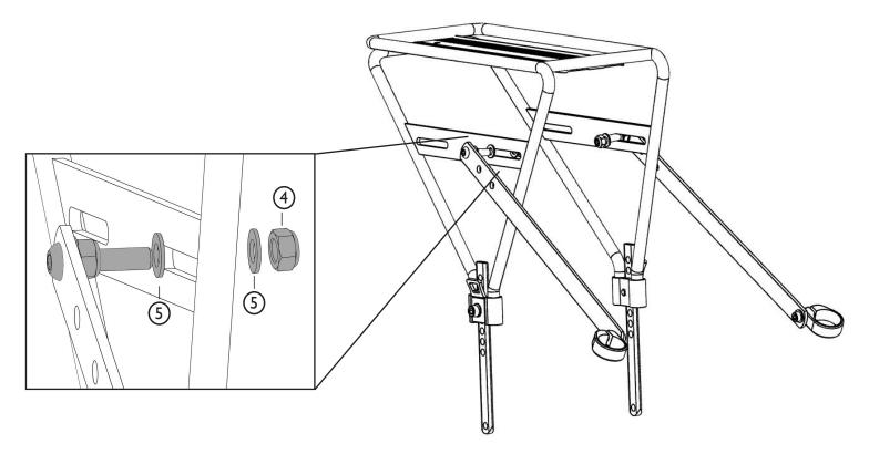
Loosen seat stay quick release levers and detach upper seat stays from lower seat stays. Loosen seat stay quick release set screws and remove clamps.
