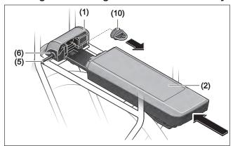
In order for the battery to be inserted, the key **(5)** must be inserted into the lock **(6)** and the lock must be open.
