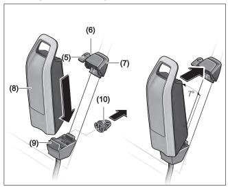
In order for the battery to be inserted, the key **(5)** must be inserted into the lock **(6)** and the lock must be open.
