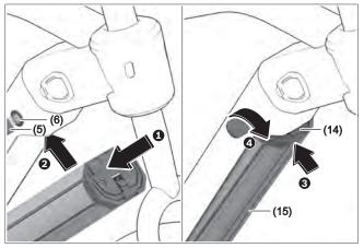
In order for the battery to be inserted, the key **(5)** must be inserted into the lock **(6)** and the lock must be open.
