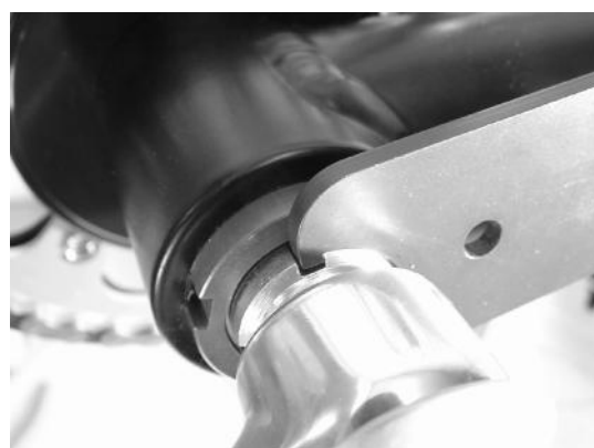
Fig. 8: Adjusting of gearing play. No preload!
