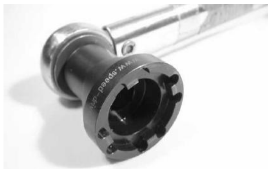
Fig. 5: Use the box wrench in combination with a torque wrench.
