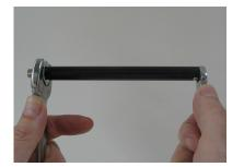
This photograph shows the inner end of the Quick Release rod projecting from the inner end of the axle after the button has been released. This means that the balls are partly depressed, and the wheel may come off in riding. If this is the case with your trike, please adjust it, or have a Dealer adjust it for you.
