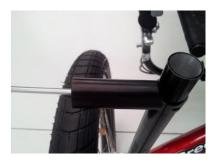
Note that the angle of the mudguard to the wheel in the vertical plane can be adjusted by rotating the clamp rearwards around the kingpin, and in the horizontal plane by rotating the Accessory Mount around the post. The mudguard can also moved up and down on the post, and and in and out on the Accessory Mount. Finally the mirror can be mounted on top of the post:
