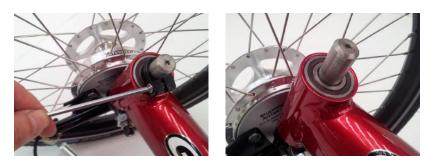
Then fit the mirror post clamp with the widest web between the two holes up, so that the mirror post will sit more vertical than the kingpin:
