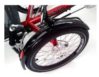
Also note that the mudguards should be positioned well clear of the tyres to allow for mud and stone clearance as shown:
