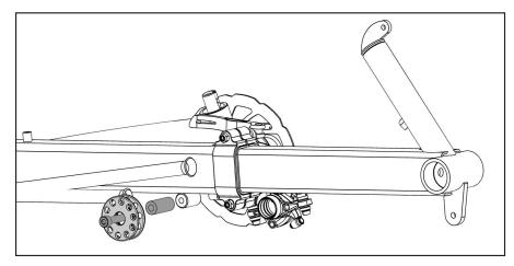
Install Moving Idler Rod Assembly on boom mount using the M8x35 bolt (4) and M8 Nyloc Nut (3).
