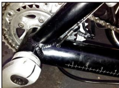
Putting Front Derailleur Cable Through Crank Extension
