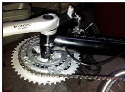
Putting Front Derailleur Cable Through Crank Extension
